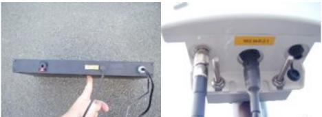
Left: Encoder unit, shown out of rack. Note ethernet cable plugged into jack. Right: Transmitter / Receiver. Note Rotary ethernet cable attached in the middle.
