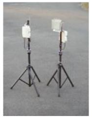
Photo: Omnidirectional Link Kit (left) and Directional Link Kit (right)
