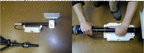
Finally take the provided outdoor Ethernet cable (dark grey, standard ethernet jack on one end, rotary connector on the other end), and plug it into the standard Ethernet jack on the back of the Encoder unit in the Output Pack Control Rack. Then take the other end of the cable, and carefully attach it to the jack on the bottom of the white transmitter / receiver unit. Note that you plug the cable into the jack, and then rotate the locking collar to hold it permanently in place.
